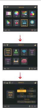
Address: 001-512; Lost status: Hold/Delay DMX status: On/Off; RDM status: On/Off Mode (16 kinds): P1.CCT&rgbw 8bit/P2.CCT 8bit/ P3.CCT&HSI 8bit/P4.rgbw 8bit/P5.HSI 8bit/ P6.CCT&rgbw 16bit/P7.CCT 16bit/P8.CCT&HSI 16bit/ P9.rgbw 16bit/P10.HSI 16bit/P16.GEL V2 8bit/ P17.GEL V2 16bit/P18.x.y 8bit/P19.x.y 16bit/P22.Effect 8bit/ P23.Effect 16bit/P24.LE CCT&RGBW 8bit/P26.LE HSI 8bit P30.Ultimate DMX 8bit
