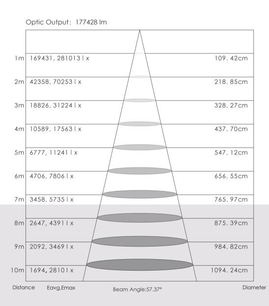
Remarks: The curve shows the irradiation area and average illumination per various irradiation distance for the lamp
